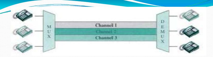
Transmission path is divided into three parts, each representing a channel to carry one transmission.
